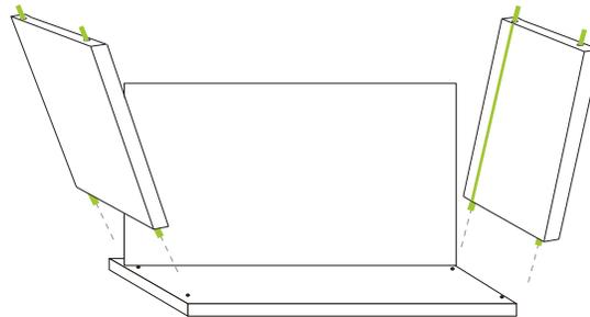
**4** Arrange vertical zBoard with grooves facing backboard as shown.
