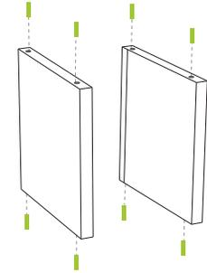
**3** Place alignment pins in vertical zBoards.
