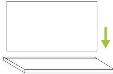
**1** Fit backboard into horizontal zBoard groove.
