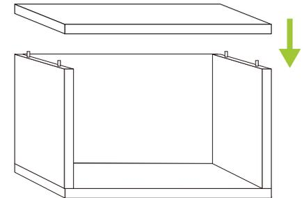
**6** Align horizontal zBoard and press firmly to secure unit together. Visit links below for more details.
