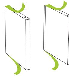
**2** Carefully remove the 3M protective layer from adhesive.
