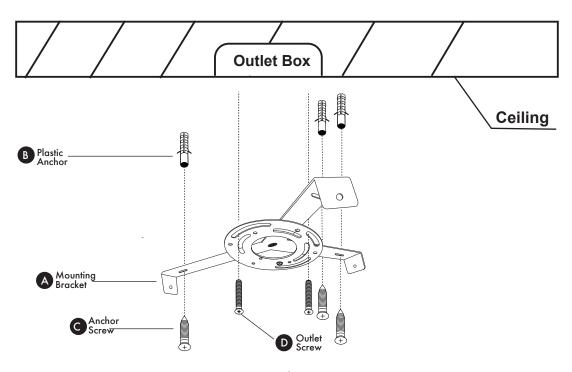
Attach mounting bracket (A) to outlet box with outlet screws (D). Screw anchor screws (C) into plastic anchors (B) to secure mounting bracket (A).
