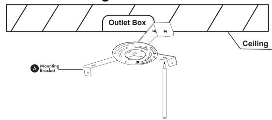
Remove mounting bracket (A) from fixture. Raise mounting bracket (A) to the ceiling. Mark location for the plastic anchors (B). Drill holes for plastic anchors (B). Insert plastic anchors (B) into hole.
