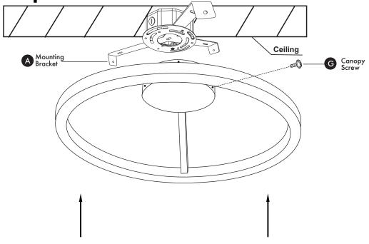
Attach fixture to mounting bracket (A). Secure fixture with canopy screw (G).
