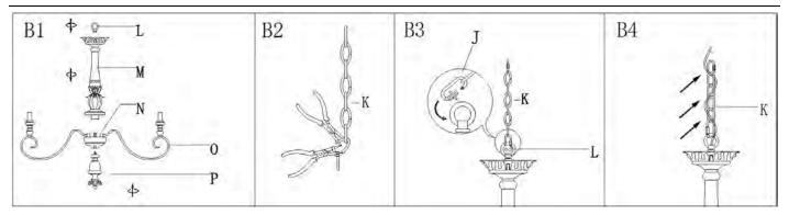
Step B1: Thread the post (M)onto the fixture body (N) till snug; thread the loop (L)onto the post (M) till snug; thread the finial (P)onto the fixture body (N) till snug.
