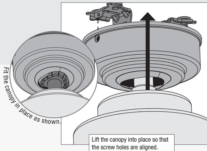
Lift the canopy into place so that the screw holes are aligned.
