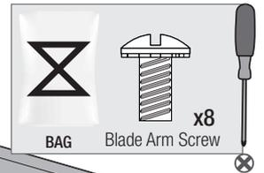
Lightly attach the blade arms to the motor with screws found in the
