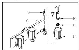
Step.4: Install G9 LED bulb(G) into socket, Position Glass(F) onto the socket of fixture body(C), then secure with socket ring(D) with Glass (F) onto Fixture body(C) by using spanner(E). Page 2 of (2)
