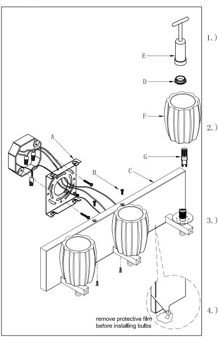
Step.1: Fasten the mounting bracket(A) onto the outlet box using two outlet box screws.
