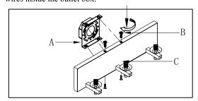
Step.3: Place the fixture body(C) against mounting bracket, Align the two holes of the mounting bracket and fixture body, then tighten the screws(B).
