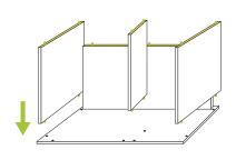
Align vertical zBoards to horizontal zBoard as shown. Press down firmly.
