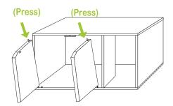
Orient door properly as shown and align bottom pin. Press on spring loaded top pin and insert.
