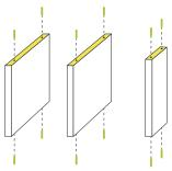
Insert alignment pins to side zBoards and middle zBoard.
