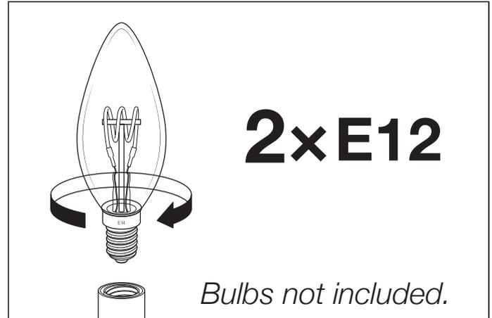
5. Carefully place the bulbs in the fittings. Do NOT turn the bulbs further than necessary, to prevent damage to the fitting.
