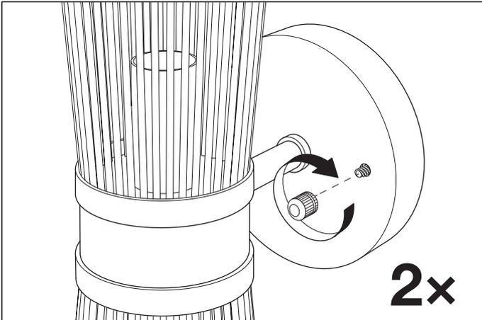
3. Fix the lamp securely with the knobs.
