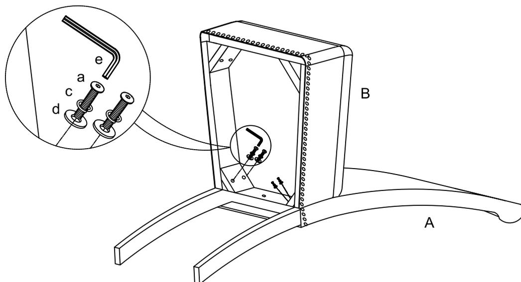
Step 3. Attach front legs (C) to seat cushion (B) using bolts (b), lock washers (c) and flat washers (d). Loosely tighten the bolts with Allen wrench (e).
