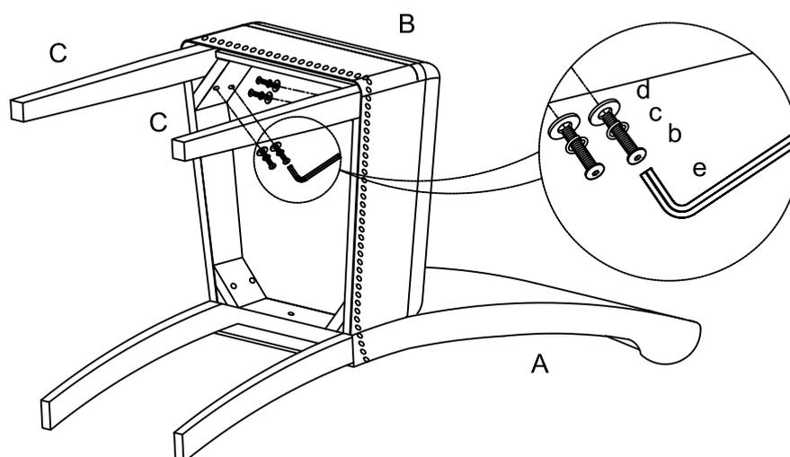
Step 4. Securely tighten all bolts by allen wrench (e), but do not over tighten the bolts. Assembly is complete.
