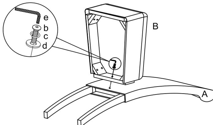
Step 2. Attach seat cushion (B) to chair back (A) using bolts (a), lock washers (c) and flat washers (d). Loosely tighten the bolts with Allen wrench (e).
