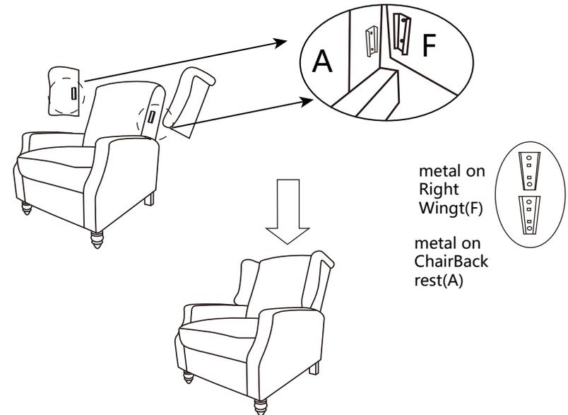
**STEP 6:**Insert the small metal on the sides of the Left and Right Wing(E)(F) into the prefabricated slide lock gadget on the Chair Backrest(A) as shown above. Firmly but gently,push the Wing downwards until the Wing is fully slotted and locked into position.
