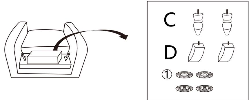
**STEP 2:** Remove the small carton and take out the Front Legs(C), Hind Legs(D) and Gaskets(①)
