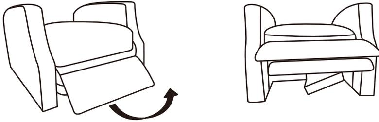
**STEP 3:** Pull the front footboard away from the front of the Chair Base (B). And you can see the Left Wing (E) and Right Wing (F) in the Chair Base (B).
