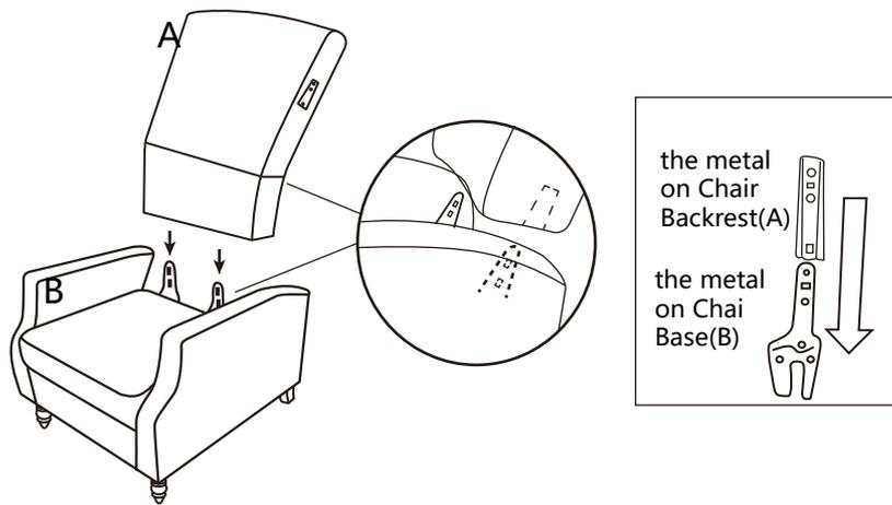
**STEP 5:**With assistance of your adult partner,hold up the fully assembled Chair Base(B). Insert the small metal arms on the sides of the Chair Backrest(A) into the prefabricated slide lock gadget on the Chair Base(B) as shown above. Firmly but gently ,push the Chair Backrest(A) downwards until the Chair Backrest(A) is fully slotted and locked into position.
