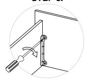
Step1--Loosen screws on back of drawer front brackets as shown.
