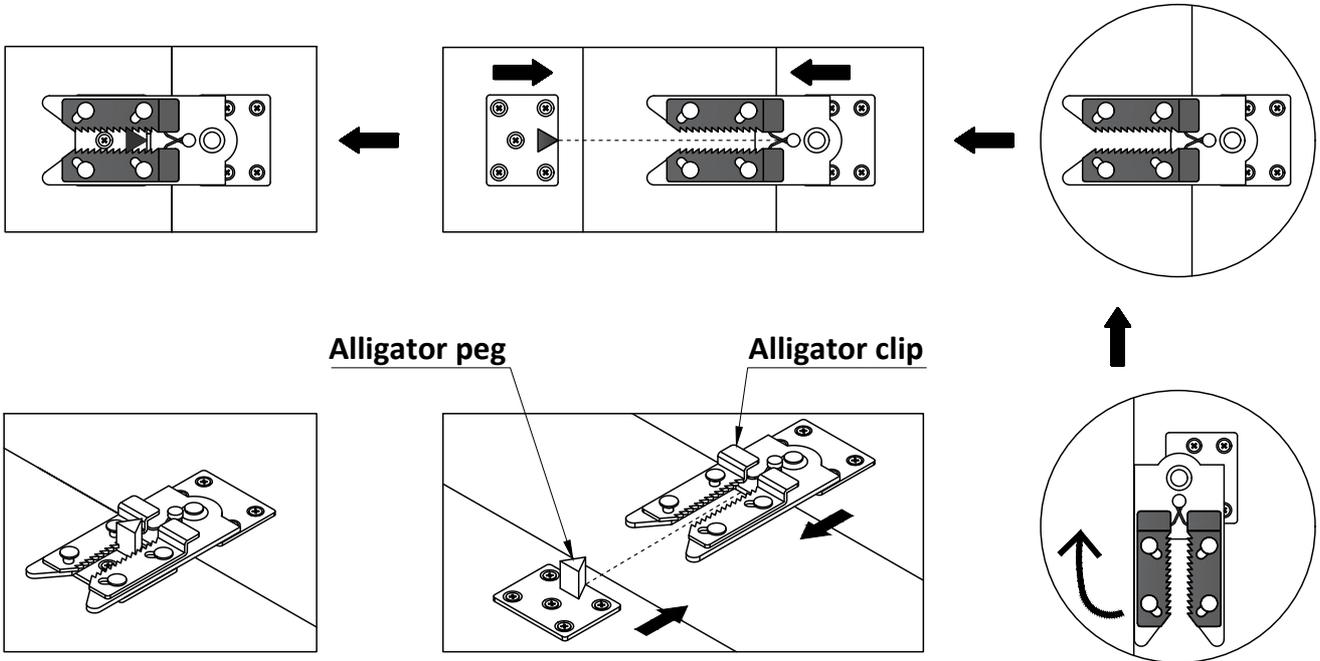
Rotate the connector clip 90 degrees.
