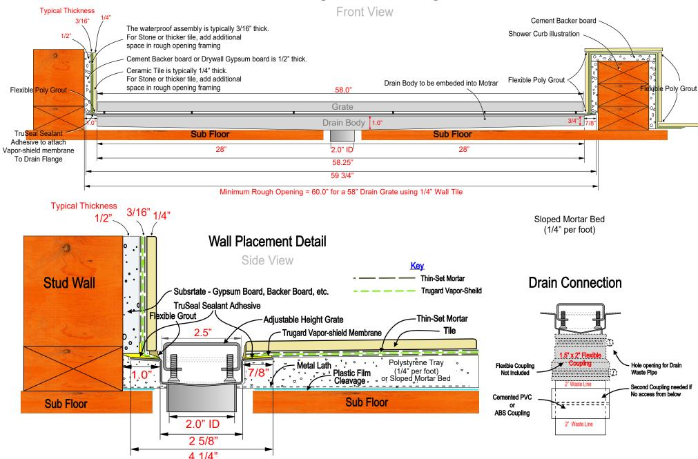
Note: To determine the framing rough opening size, add one inch to the length or width of the drain body, if a one quarter inch thick tile is being used. If the tile or stone is thicker than the 1/4" and the additional thickness of the tile to the 1 inch distance normally used to determine the rough opening size. So for example, for the rough opening for a 70 inch linear drain, the rough opening would need to be 72 inches, when 1/4" tile is being used.
