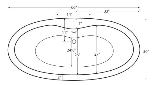
Features a 7" wide flat deck surface on the drain side for mounting faucetry.
