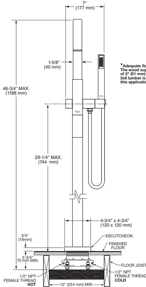
\*Adequate floor support is required. The wood support must be a minimum of 2" (51 mm) thick by 10" (254 mm) wide. 2x6 lumber is NOT adequate for this application.
