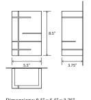
Dimensions: 8.5" x 5.5" x 3.75" Materials: solid wood, polymer Product weight: 4 lb Light source: integrated LED Light output: 1130 Lumens (source) Light color: 2700 K or 3500 K Color accuracy: 90+ CRI Power usage: 13 W Dimmable (see driver below) Wood grain will vary Specifications subject to change
