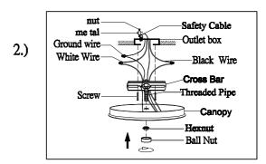
Step.2: Remove mounting bracket from fixture and install to electrical box. Wire fixture to wires in outlet box. Copper wire is for Ground. On wire side
