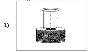
Step.3: Install fixture to bracket and tighten screws at the ends of the canopy (D) to secure.
