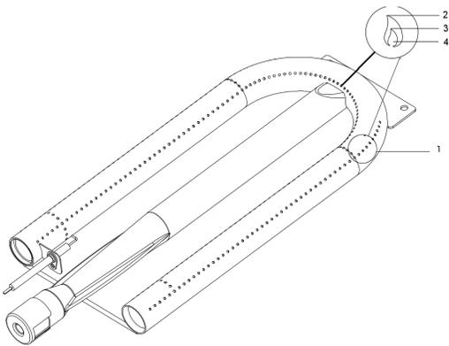
The factory burners have been set for the correct air and gas mixture. The correct flame pattern is shown in the figure to the left. Please inspect at each and every use.
