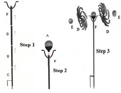
**Step 1**- Attach the stake parts (C), 2x (B), and (F) by screwing each one into each other. Start with (C) and end in (F). See Step 1 above.
