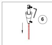
**6** Tighten top set screw first, then lower set screw snugly. Smooth out any bulges in braided wire.
