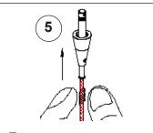
**5** Feed inner wire into quick connect adapter until it reaches top set screw. Feed braided outer wire and brass collar into quick connect.
