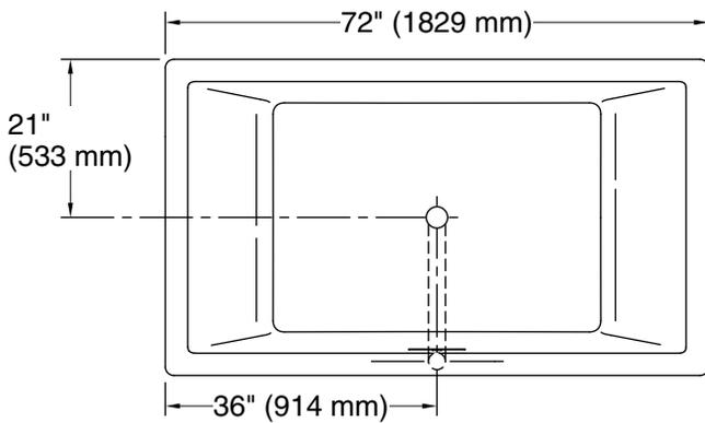
No change in measurements if connected with required drain illustrated. (K-7272)
