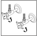
(8) Connect hot and cold inlet supply hoses to supply stops. For supply stop with 1/2" outlet connection, use 3/8" male to 1/2" female adapter for installation. Adapters are optional and are not provided with the faucet. Turn on both side supply stops to check any leaks.
