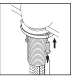
(5) Thread locknut onto the faucet shank from underneath the sink. Position faucet to desired location from the top and hand-tighten locknut till it won't go further. Thread both screws on locknut and tighten screws on locknut with the help of a Phillips head screwdriver to secure faucet. (Note: Do not overtighten.)
