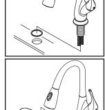
(3) For 3-Hole Installation:- Install supplied deck plate underneath of the faucet. Apply plumbers putty under the base gasket. Place the faucet in position on the sink.
