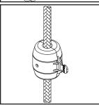
(7) Install weight on spray head hose. Adjust weight's position so the spray head can be retracted properly.
