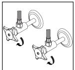
(1) Shut off the water supply. Remove old faucet. Clean mounting surface in preparation for new faucet.
