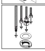
(4) With flat side of the locknut facing down and the steel washer inside the locknut please follow the order as the drawing shows to insert flex hoses through the center hole of the locknut from underneath the sink.
