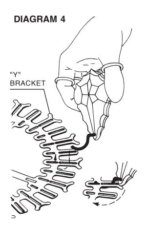
Position the crystal above the "Y" bracket so that the end of the hook enters the long slot, gently push toward the center of the fixture and raise the crystal making sure that the end of the hook comes up through the short slot, in line with the long slot.
