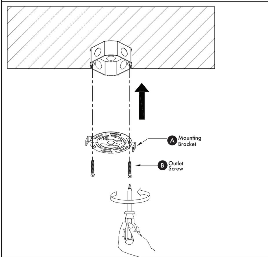
**Secure mounting bracket (A) with outlet screws (B).**
