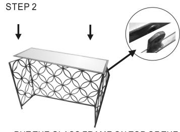
PUT THE GLASS FRAME ON TOP OF THE BODY PANEL CORRESPONDING THE HOLES TO THE HOLES
