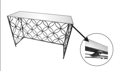
PUT THE SCREWS IN THE CORRESPONDING HOLES AHD TIGHTEN IT WITH A WRENCH
