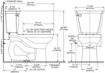
NOTES: THIS TOILET IS DESIGNED TO ROUGH-IN AT A MINIMUM DIMENSION OF 305MM (12") FROM FINISHED WALL TO C/L OF OUTLET. SUPPLY NOT INCLUDED WITH FIXTURE AND MUST BE ORDERED SEPARATELY. \* DIMENSION SHOWN FOR LOCATION OF SUPPLY IS SUGGESTED.
