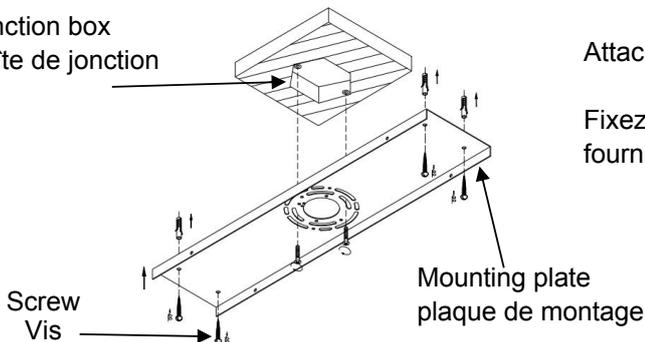
Attach the mounting plate to junction box with screws provided.
