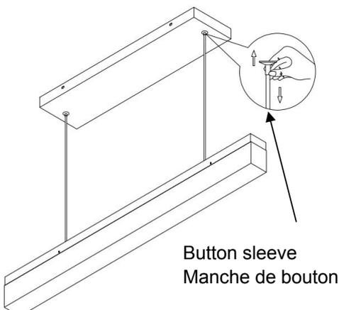
Before installation to ceiling, adjust fixtures to desired length by pushing wire up into canopy, then coiling up excess wire, minor adjustment can be made after installation. To lower or lengthen wire, depress button sleeve located where wire comes out of canopy.
