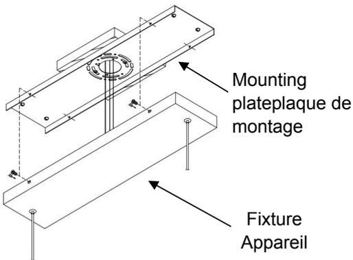
Attach the fixture to the mounting plate with screws provided.
