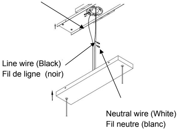
Connect the GROUND WIRE from junction box to GROUND (COPPER or GREEN) wire from fixture with a wire nut. Connect the NEUTRAL WIRE from junction box to NEUTRAL (WHITE) wire from fixture with a wire nut. Connect the LINE WIRE from junction box to LINE (BLACK) wire from fixture with a wire nut.
