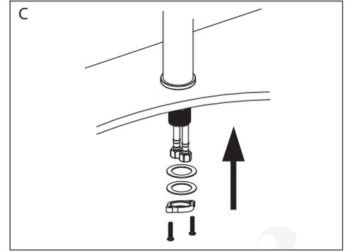
C. From under the sink, install the rubber washer, steel washer and locking nut onto the shank. Tighten the locking nut and install the 2 screws to secure the faucet in place.
