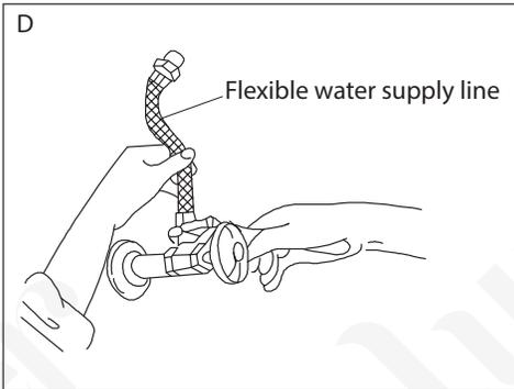
D. Use an adjustable wrench to tighten the water supply hoses. (**IMPORTANT:** Do not overtighten the connections.)
