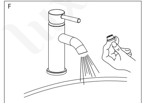
F. Remove the aerator with a small coin or a flat head screwdriver and let the water run for about 1 minute to clear any debris in the plumbing system. Check for leaks at all connections. Reinstall the aerator to complete the installation.
