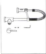
m off water and relieve pressure! Detach handle button mg a small flathead screwdriver, unscrew set screw mg Allen Wrench and take off handle.
