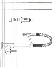
After installation is complete, remove aerator and rotate handle to the closed position. Turn on the water supply valves, and check all connections for a leak. Turn on your faucet and allow both hot and cold water to run alleast one minute each. Replace Aerator.
