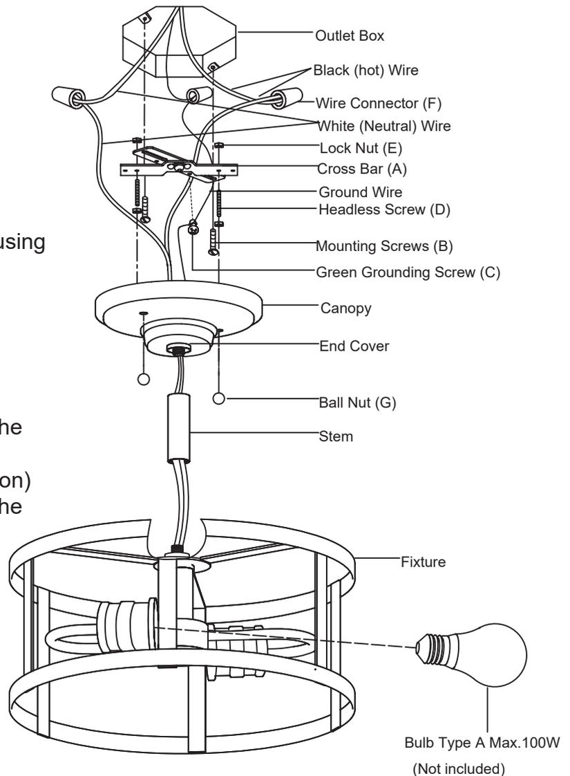
6. Put the fixture in the canopy, tighten with headless screws and then secure it with two ball nuts.
