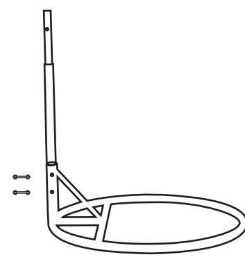
**1.put the base on the ground and remove the package.**
