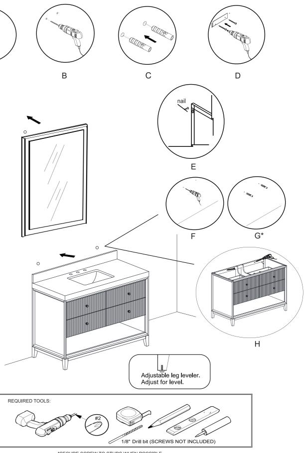
\*SECURE SCREW TO STUDS WHEN POSSIBLE
