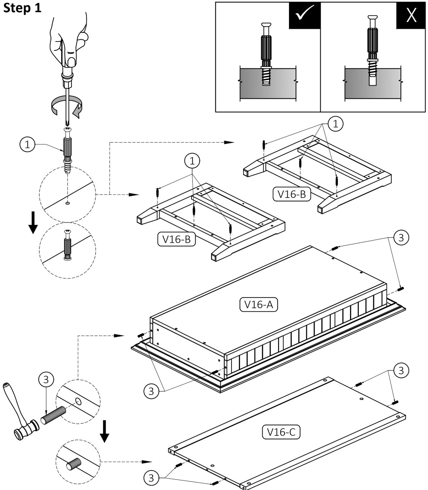
1. Attach three Cam Lock Pins ① into pre-drilled holes on each Side (V16-B).
