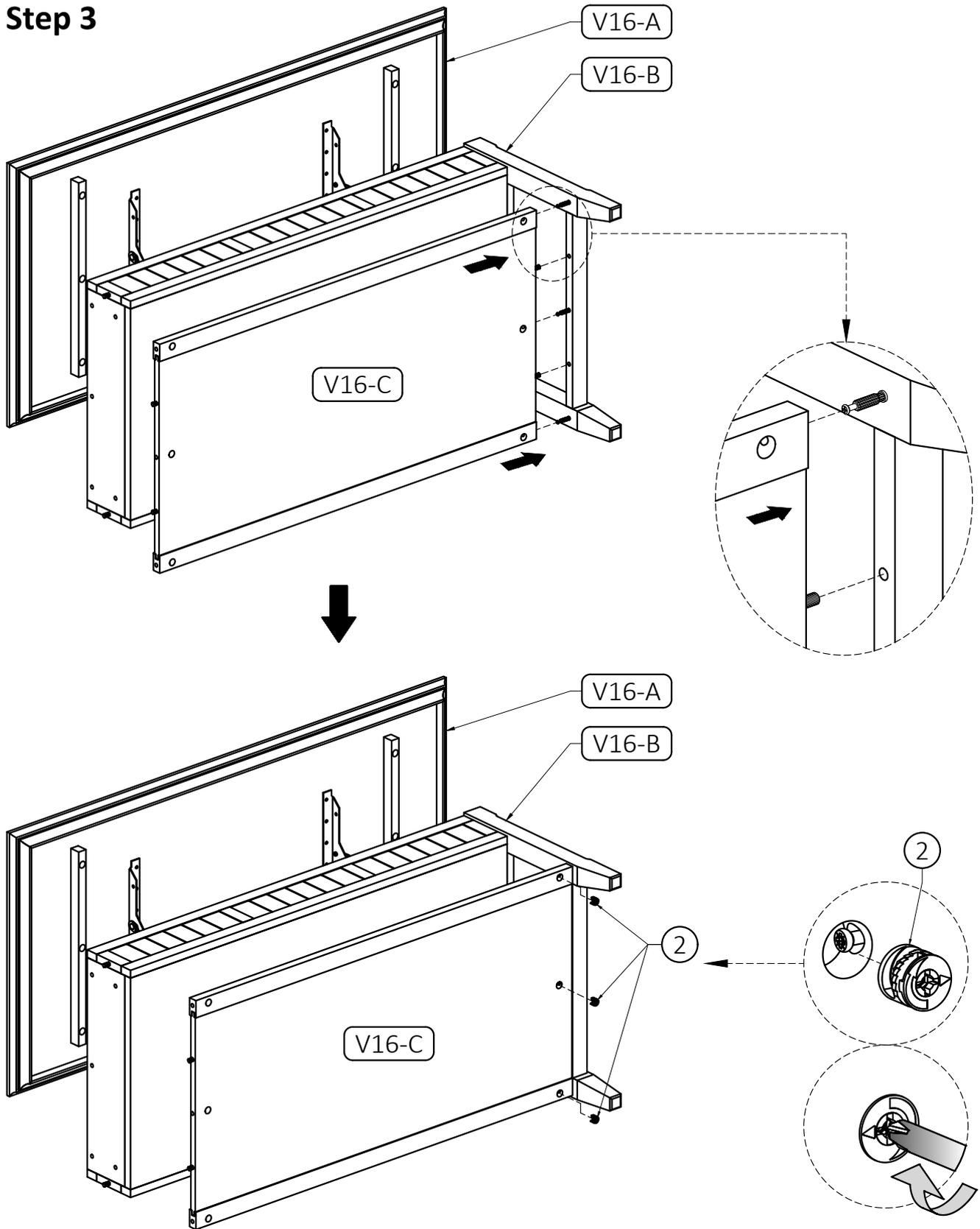
1. Align Cam Lock Pins and Wood Dowel with guide hole and attach Bottom Shelf (V16-C) to Side (V16-B).
