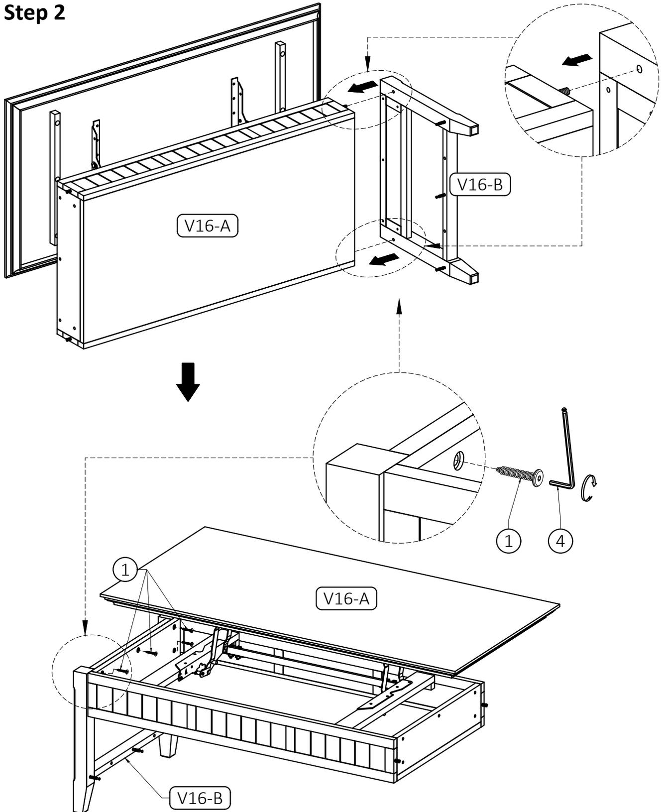
1. Align Wood Dowels with guide holes and attach first Side (V16-B) to Top (V16-A).
