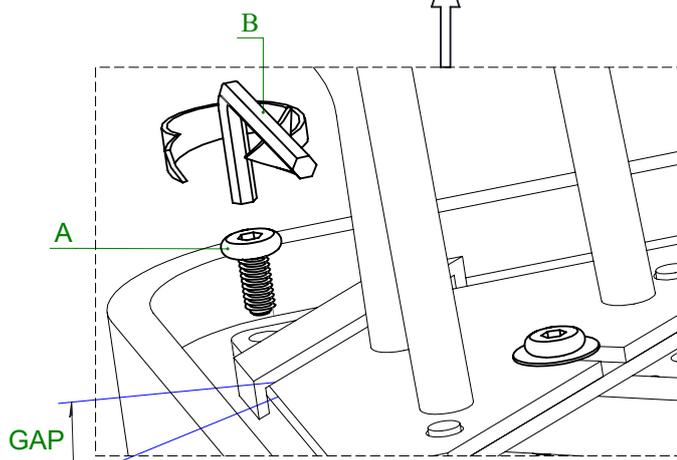
TIGHTEN BOLT COMPLETELY.
