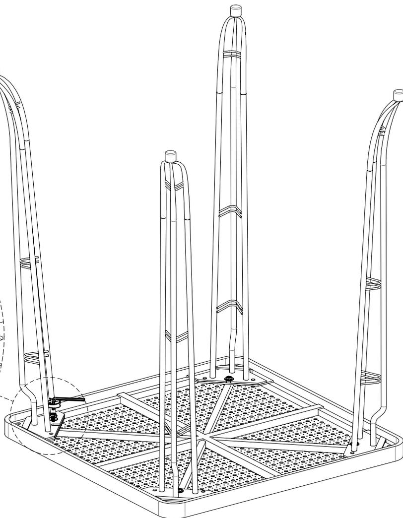
DO NOT TIGHTEN BOLT COMPLETELY.
