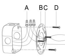
Step 1:Connect the mounting plate (B) to the junction box using the mounting screws (D).
