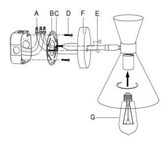
Step 3: Fix the lamp body (F) to the mounting plate (B) with nuts (E). Then Step 4: You can adjust the lampshade left and right, up down. insert the bulb (G) into the lamp body (F).
