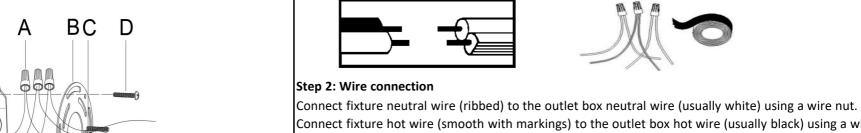
Connect fixture hot wire (smooth with markings) to the outlet box hot wire (usually black) using a wire nut.
