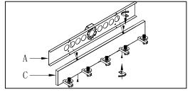
Step.3: Place the fixture body(C) against mounting bracket, Align the two holes of the mounting bracket and fixture body, then tighten the screws.
