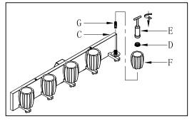
Step.4: Install G9 LED bulb(G) into socket, Position Glass(F) onto the socket of fixture body(C), then secure with socket ring(D) with Glass (F) onto Fixture body(C) by using spanner(E).
