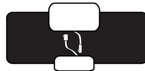
1. Insert the black wire and white wire from the light kit assembly through the hole in the gasket and the bottom of the lower switch housing. Refer to Figures 2.
