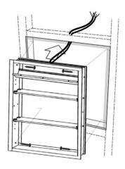
6. Insert and secure the cabinet; hardwire the power cord according to local electrical codes. You may hardwire both cables to the same power supply. Connect the wall switch to the white cable (Main) if one is used. A separate power supply is required for the Outlet (black cable).
