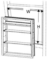
4. Frame out the wall cavity so the cabinet fits tightly into the recess.
