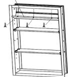
2. Loosen the electrical enclosure Cover Plate by removing the 3 screws and pivot down the Cover Plate.
