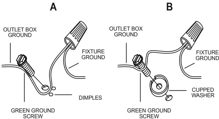
Connect wires according to the chart below
