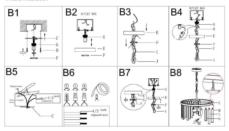
Step B1 » Remove collar ring (F) from collar loop (G). Attach single bar (C) to the outlet box with mounting screws (B).
