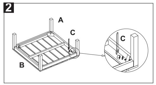
Step 2: use the Wrench (C) to tighten all legs as shown on the picture.
