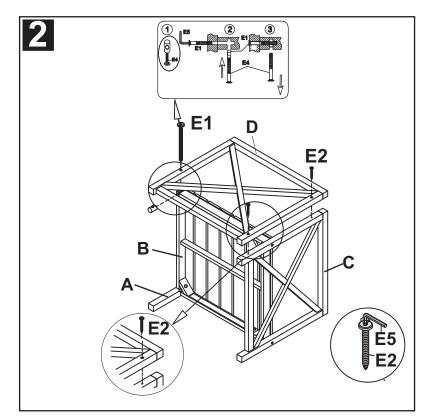
Step 2: attach the corner (D) to the chair by using the the Allen screw (E2) and the Allen Bolt (E1) and tighten both sides with the Allen Key (E5) as shown on the pictures.
