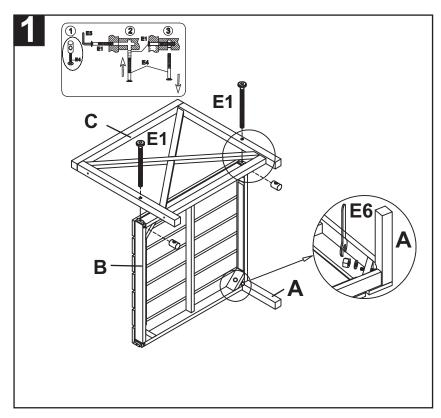
Step 1: attach the leg (A) and the back (C) to the seat (B) as shown on the picture. Then use the Allen Bolt (E1) and tighten it with the Allen Key (E5) . Then tighten the the leg (A) with the wrench (E6) as shown on the picture.
