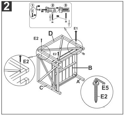
Step 1: attach the leg (A) and the back (C) to the seat (B) as shown on the picture. Then use the Allen Bolt (E1) and tighten it with the Allen Key (E5). Then tighten the leg (A) with the wrench (E6) as shown on the picture.
