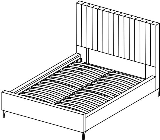
\* When moving the bed position, the center support legs must be adjust to be straight to avoid any broken problem.
