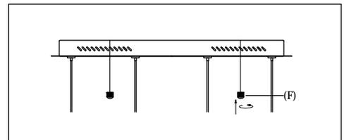
3.) **Step.3:** Adjust wire length to desired mounting height, and tighten strain relief screws to secure. Install fixture to bracket and tighten screws (F) at the ends of the canopy to secure.
