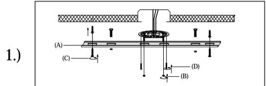
1.) **Step.1:** Remove mounting bracket from fixture and install to electrical box using screws (D). Mark where screws at ends of bracket (A) meet the ceiling. Remove mounting bracket (A) from ceiling. Drill holes using 3/16"± drill bit where marked. Install mounting bracket (A) to outlet box by attaching anchors (C) and screw nuts (B) to secure bracket at ends.
