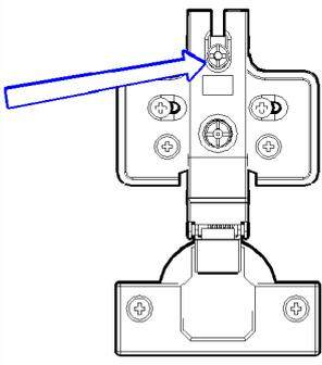
Loosen this screw, adjust by moving back and forth
