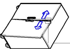
If there is a gap between the doors on the top (Please adjust slide hinge the top part door)
