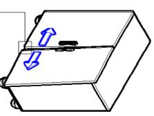
If there is a gap between the doors on the bottom (Please adjust slide hinge the bottom part door)
