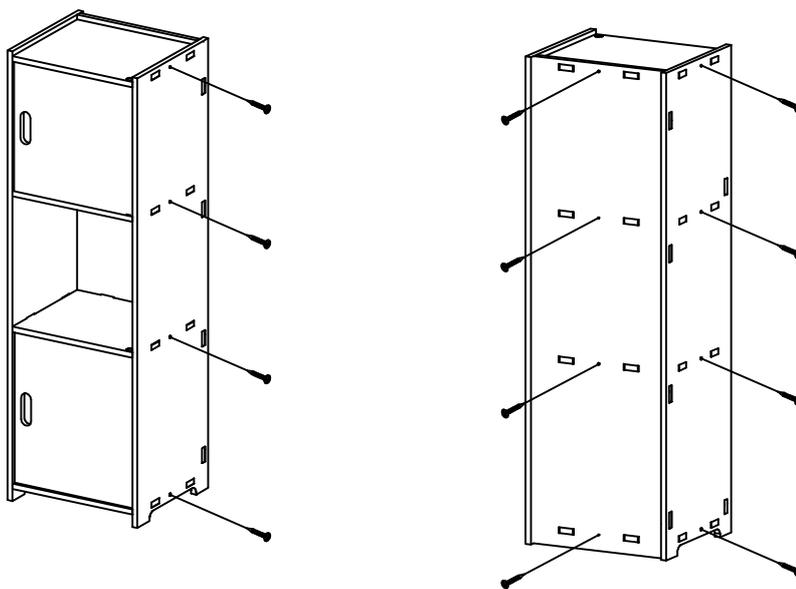
Insert and tighten unit with provided screws into pre-drilled holes to secure unit, as shown above.
