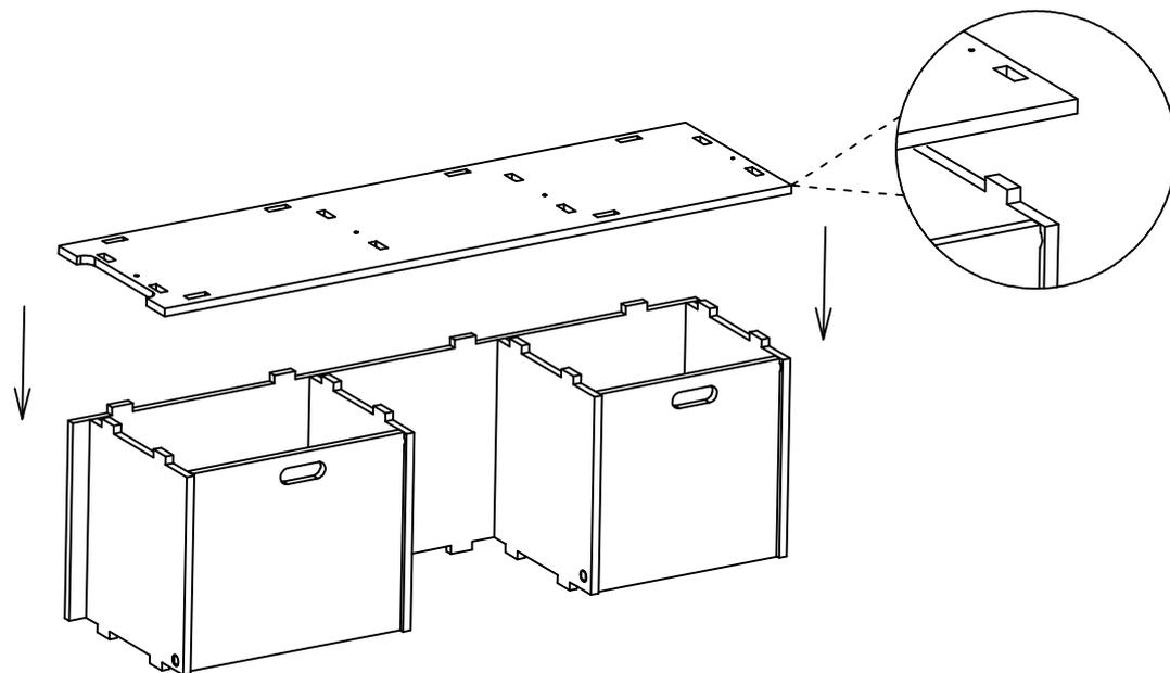
Attach the left side panel by inserting them into the pre-drilled slats.
