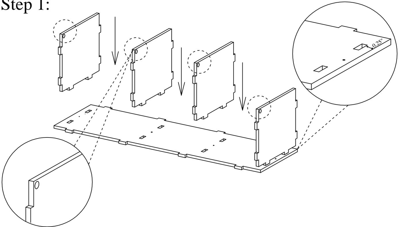
Attach the shelves to the back panel, by inserting them into the pre-drilled slats as shown above.
