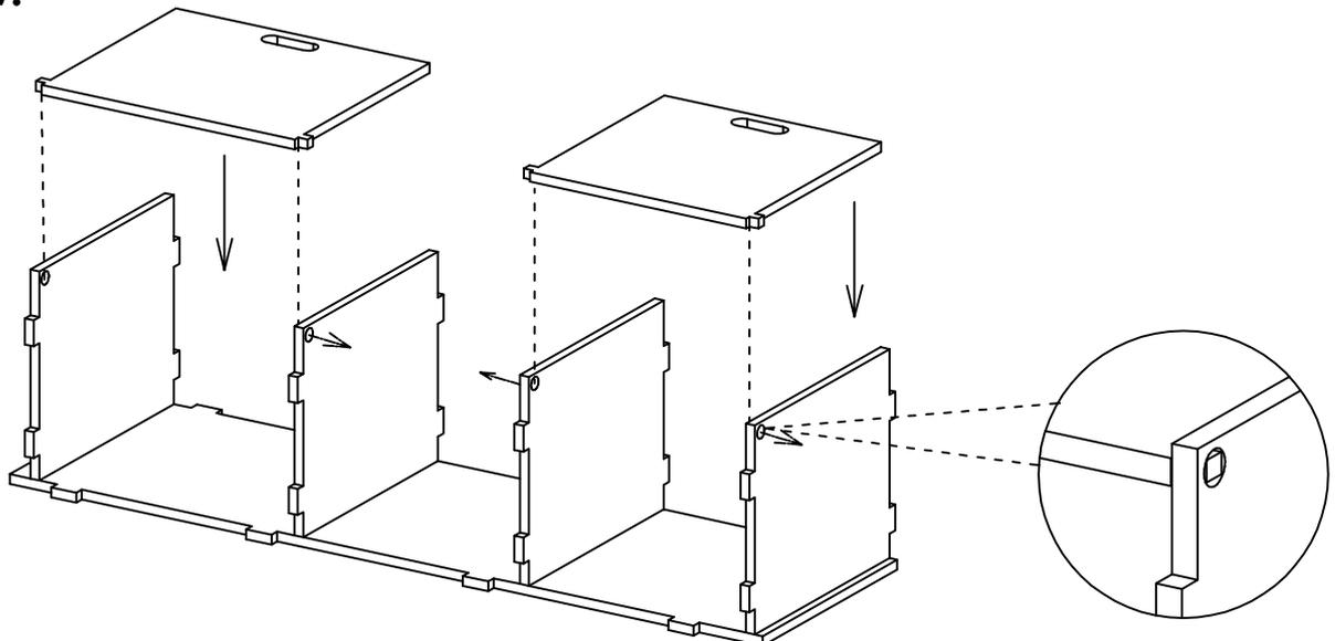
Attach the doors to the shelves, by inserting them into the pre-drilled slats as shown above.
