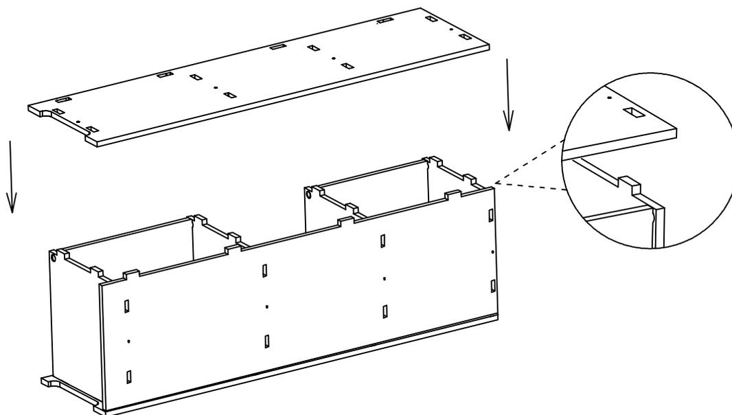
Attach the right side panel by inserting them into the pre-drilled slats.
