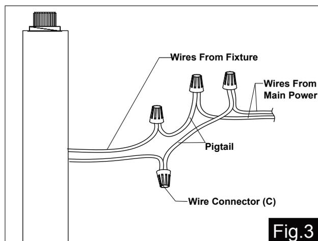
1. Turn off the power at the fuse or circuit box before starting installation.
