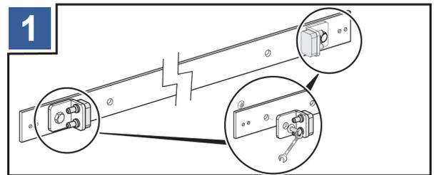
1 Before beginning installation, attach the door stops [C] to the rail [L].
