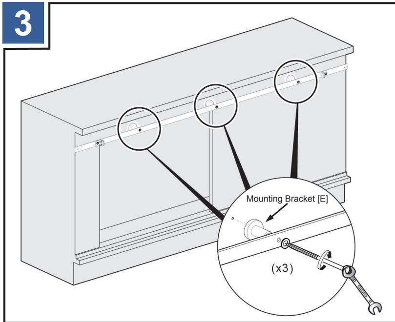
Install the rail, and mounting brackets [E].
