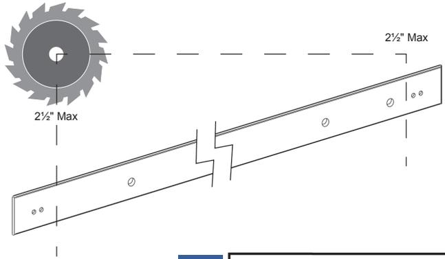
The rail can be trimmed if necessary using a band saw. Use blades suitable for iron or stainless steel depending on your rail.
