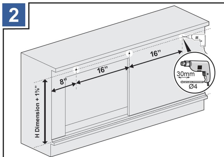
2 Using a power drill with a 4mm drill bit, drill holes as indicated.
