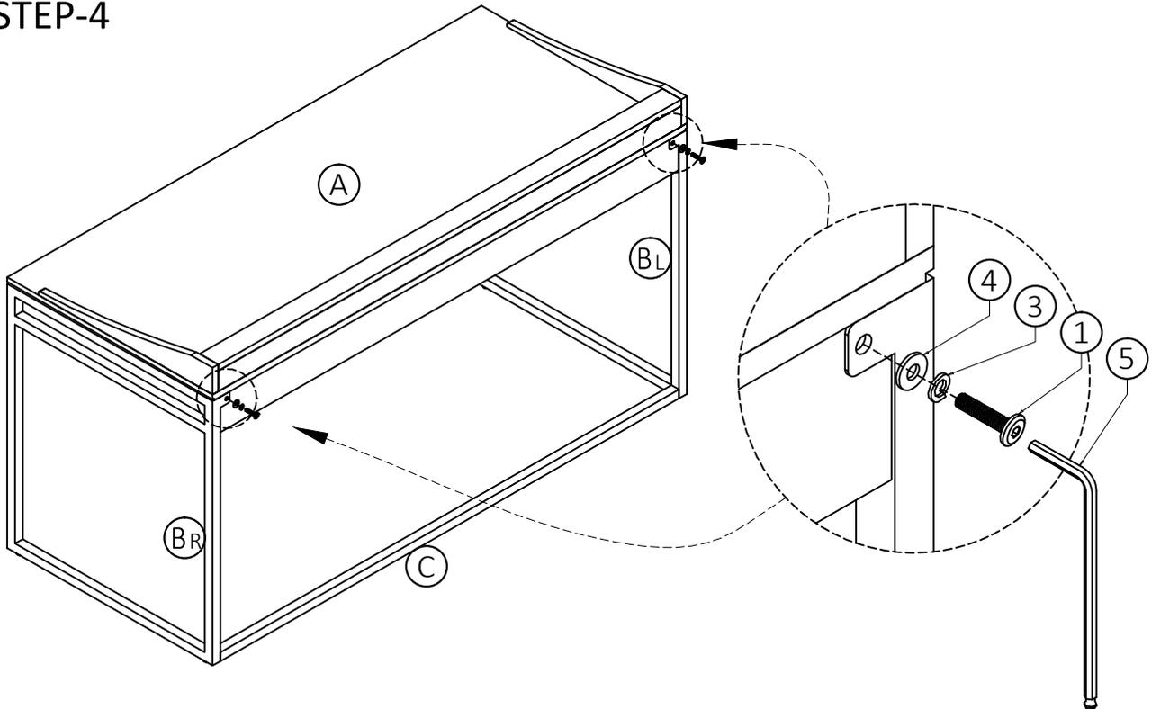
1. Use two Bolt s (1), two Lock Washers (3) and two Washers (4) to secure part (A) with (BL) and (BR).
