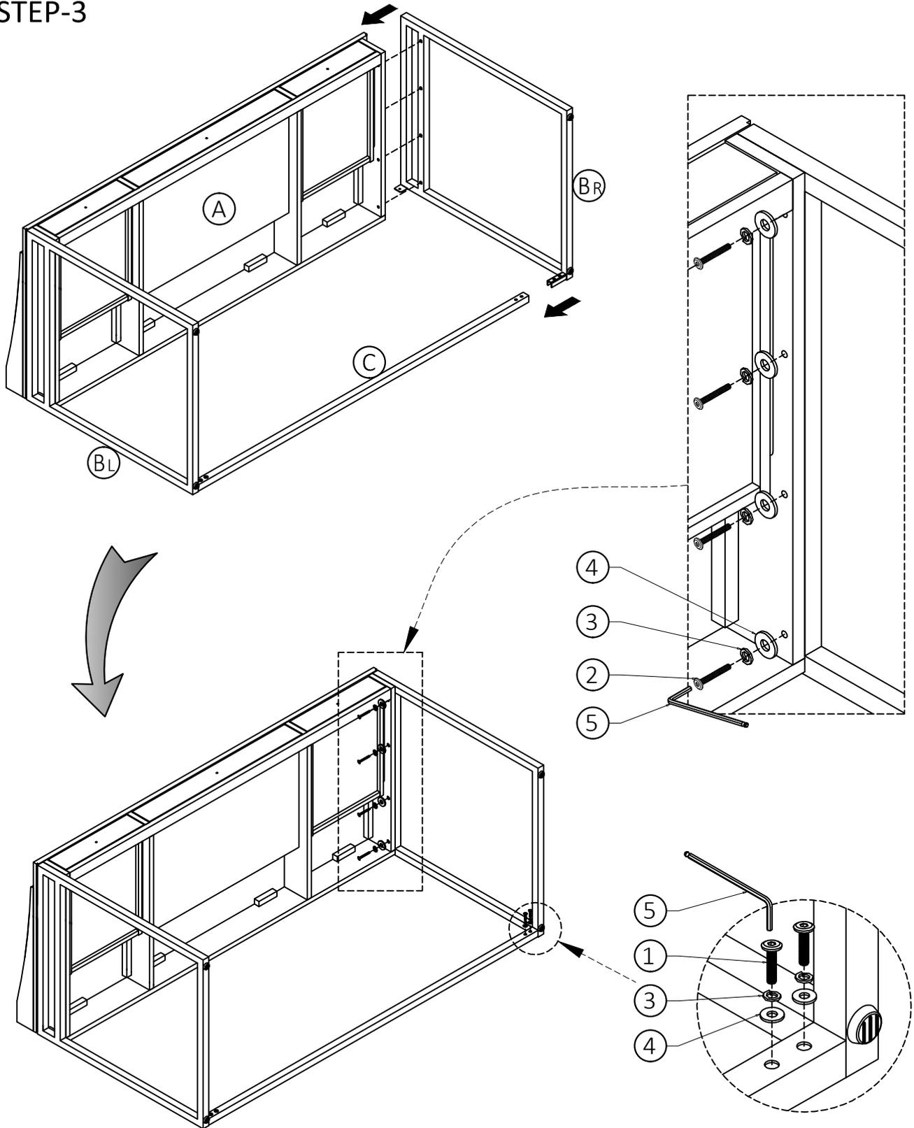
1. Align Right Side (BR) to Top (A) and Support Bar (C).
