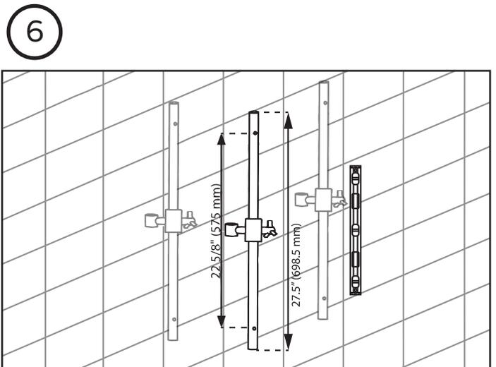
6 Hold adjustable slide bar (6) in desired mounting location. Evaluate range of adjustment and potential interference of handshower hose (15). Use level to assure shower pipe is straight.
