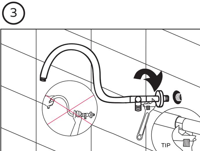
3 Insert threaded pipe into female wall fitting and tighten securely. TIP: Use diverter body to tighten by hand or use a pipe wrench on inlet piece closest to wall.
