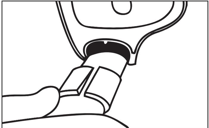
Align tab on soap dish with slot on sleeve and push soap dish down until flush. Slide lower mount (7) over slide bar and secure set screw (8).
