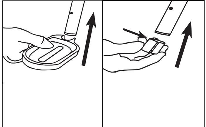
Slide ABS soap dish (12) onto slide bar followed by narrow end of tapered nylon sleeve (11).
