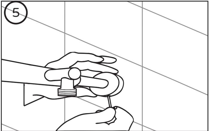
5 Secure set screw. DO NOT OVERTIGHTEN.
