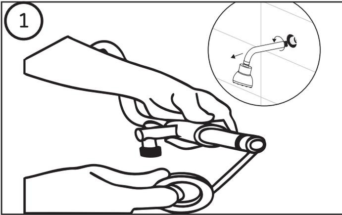
1 Remove existing shower arm and shower head. Wrap threads of shower pipe with Teflon tape and/or pipe sealant to make ensure no leaks.
