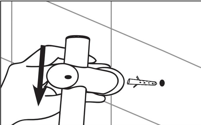
Insert wall anchors (10) until flush with wall. Slide top mount (7) over slide bar.
