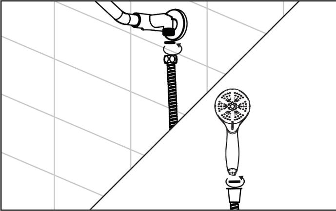
Place washer (2) in hex end of hose (15) and connect to diverter outlet.
