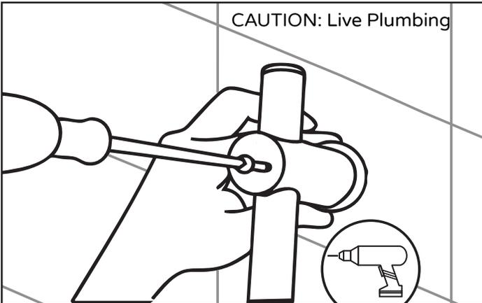
Mark wall for two mounting holes. Before drilling ensure no live plumbing can be damaged. Slowly drill 1/4" (6mm) wide by 1" (25mm) deep holes 22 5/8 inches (575mm) apart.
