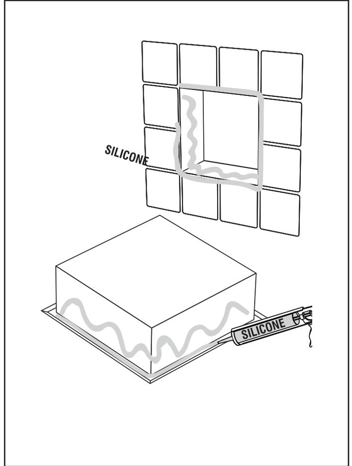
Generously apply silicone on all sides, on the inner surface of the edge of the niche, on the wall, and on the uprights (as illustrated) for optimal sealing support.
