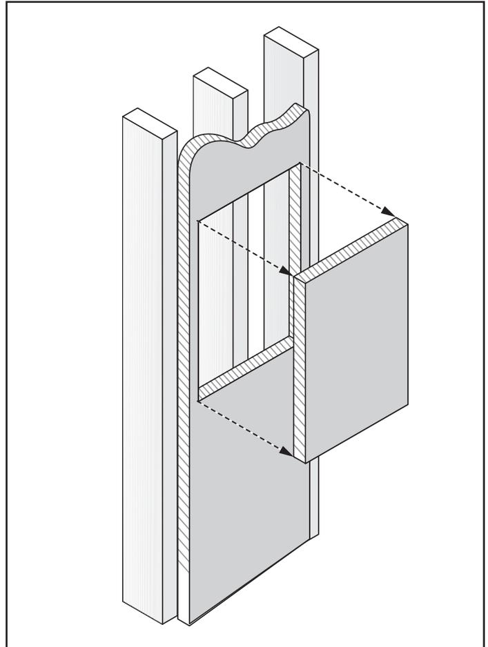
Prepare an opening between the uprights according to the dimensions X and Y of your niche, minus 1/4" (6mm). Ideally, when you insert your niche, it should offer a little resistance in the drywall to prevent it from moving until the silicone dries completely. If you have added another ceramic style finish, make it finish slightly shorter than the drywall.
