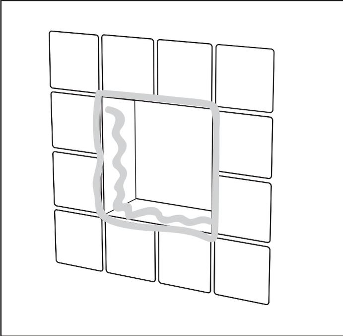
Place the niche against the wall and press firmly. Remove the niche and add silicone if it does protrude slightly.
