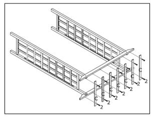
Step 3: Attach the four support brackets (Part D) to the headers (Part B) and the side lattices (Part A) as shown. Use the remaining eight screws (Hardware 2) to fasten the support brackets to the headers and side lattices.
